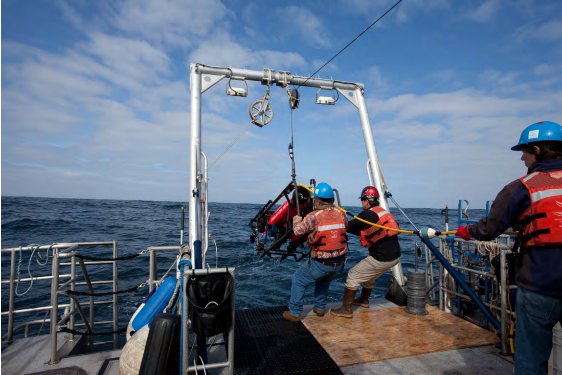
Figure 7. Recovering the ROV. Note the clumpweight has already been recovered and the tether is still being handled.
