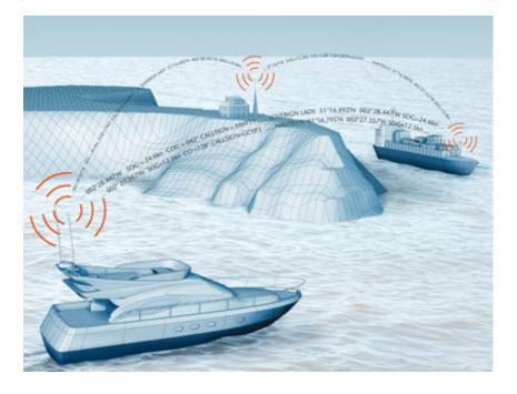
onboard device that transmits & monitors the location and characteristics of vessels in real time
