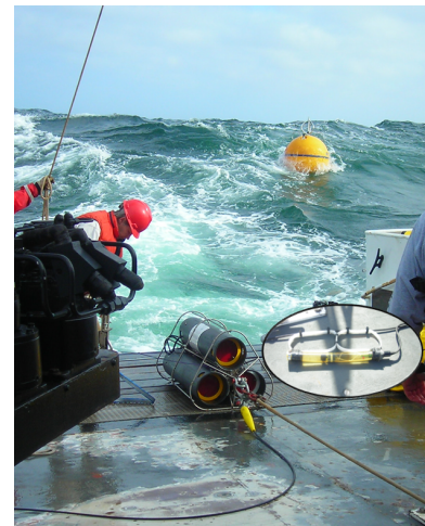
HARP deployment - high-frequency acoustic recording package
